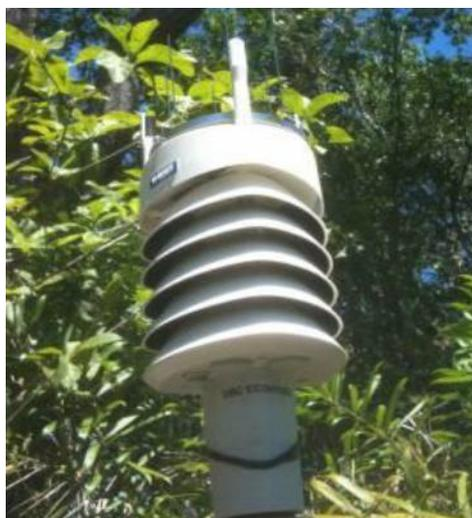
**Fig. 4** Transmissor meteorológico (modelo WXT520, Vaisala Inc., Helsinki, Finland - Brandão, 2012)
